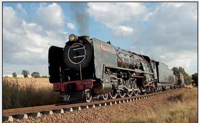
P17 - Reefsteamers normally runs their locomotives for a four-month duty cycle. (About 8 x 190km trips). Due to lack of alternative motive power in 2011/2012, this marvellous machine has been running all of our trips for just over a year. As of end March 2013, 15F No.3046 will be staged for a new 3-year boiler ticket. (Pic by A. McCarthy)
