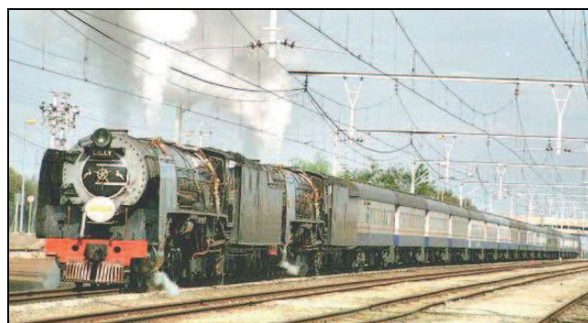
No.3472, then named 'Lilly', hauling the Trans Karoo through Oberholzer. No.3472 was one of four 25NC's kept in running order for this type of service. Notice the SATS-era coaches. She still has the unusual copper-pipe cow catcher to this day, but it is now painted black. (Pic source : Unknown)
