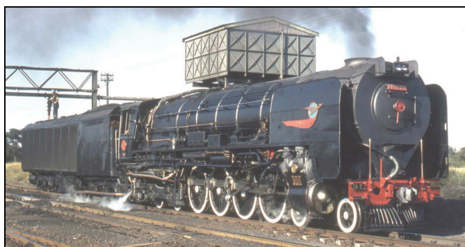
Our Class 25NC No.3472 used to look like this! Note the condensing tender with 8 radiator panels, and the unusual 'banjo' shaped smokebox. This is No.3511 'Frieda', watering at Hartswater in 1981. Only 3 of the 25s were not converted, and one of those 3 was scrapped. The locomotive pictured survives, unserviceable, in Kimberly. (Pic – Malcolm Best)
